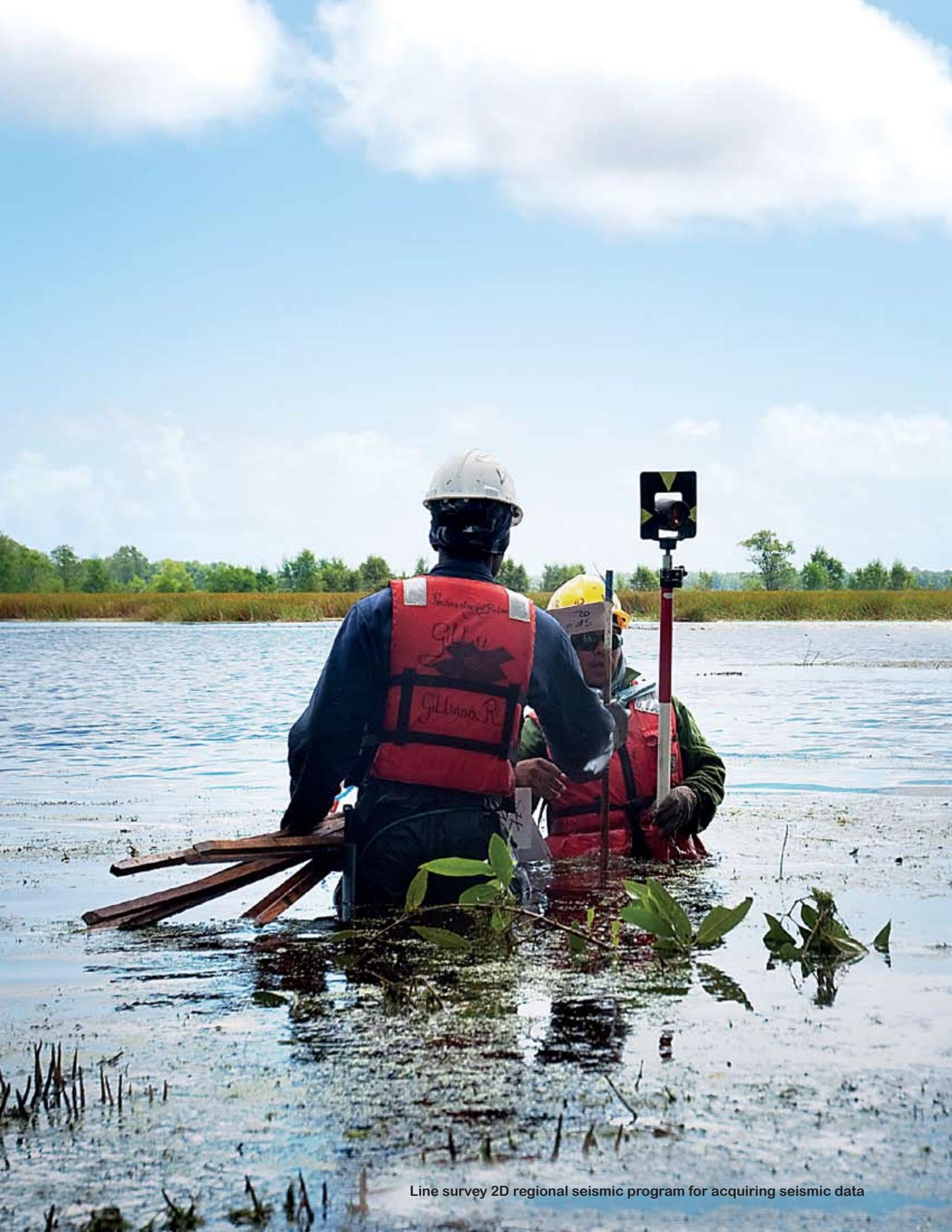
Line survey 2D regional seismic program for acquiring seismic data
