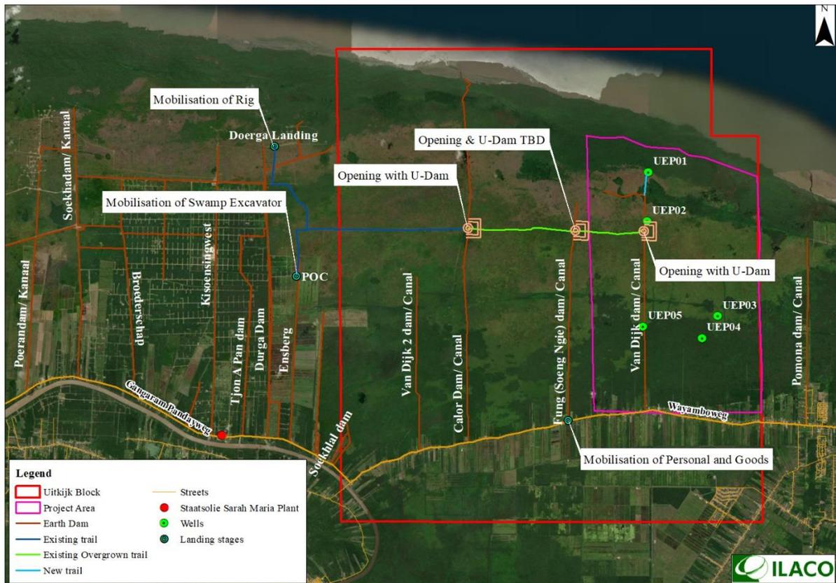
Figure 4: Overview existing trail and one new trail to be constructed and planning construction
