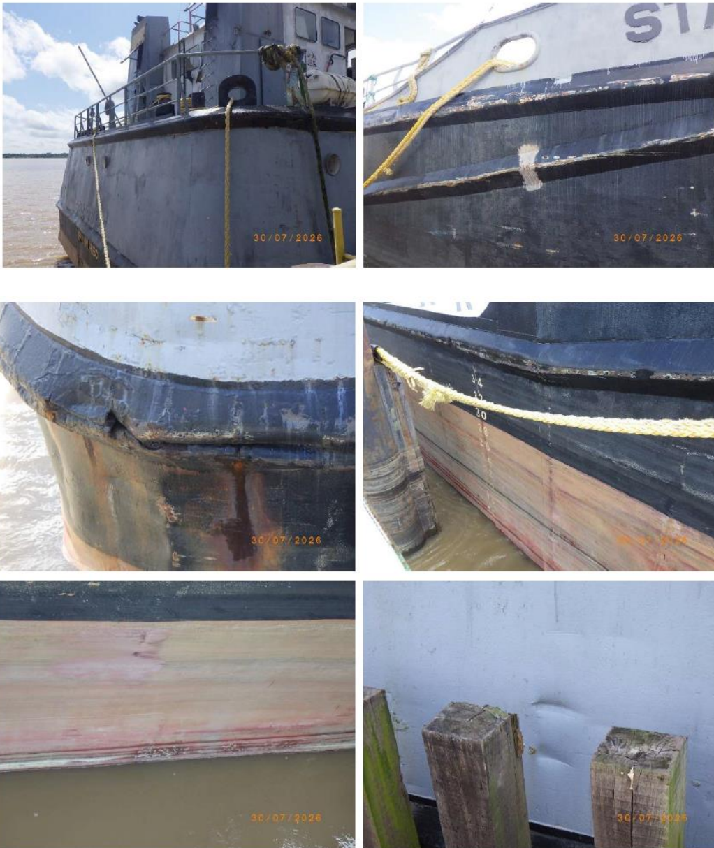
Exterior hull, port side: corrosion, defect detail deformation
